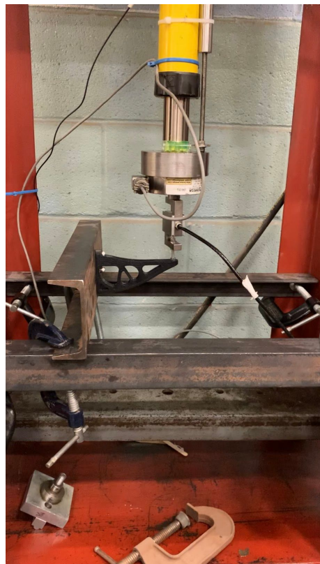
Figure 24: Test apparatus with bracket installed.
