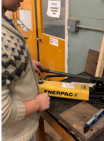
Figure 25: Lever device used to control the actuation of the hydraulic press.
